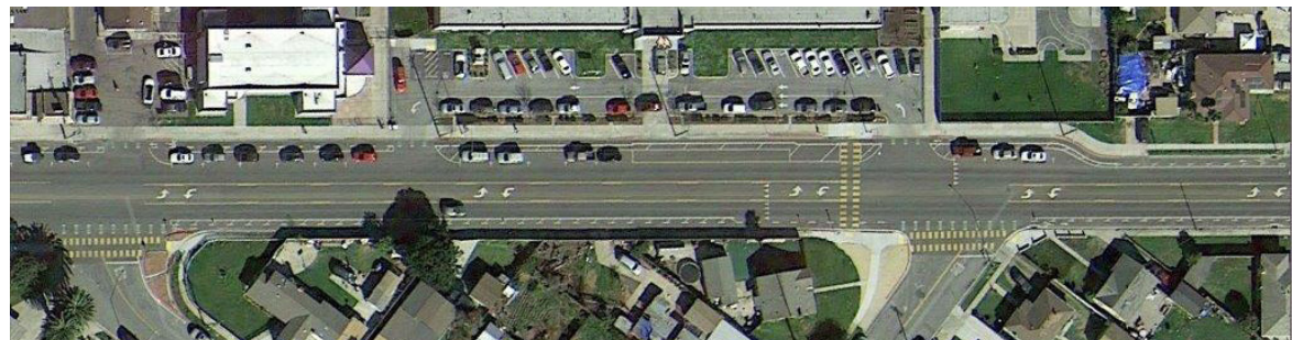
The recent Safe Routes to School project on East Market Street added traffic calming elements, bike lanes, and high-visibility crosswalks.
